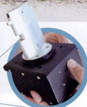
STORM SEEKERS AirDat's Tamdar sensors, currently installed on the nosecones of 160 commercial airplanes, beam real-time atmospheric data to forecasters.
